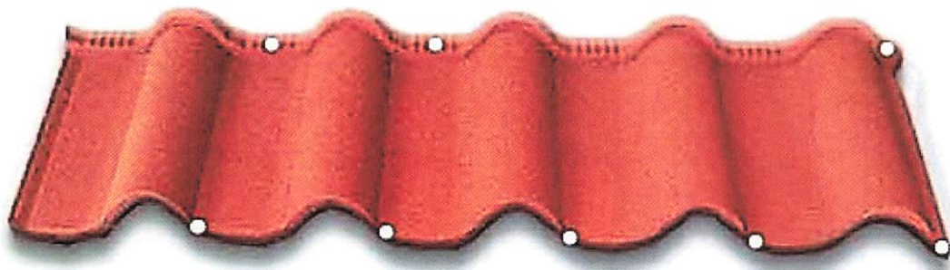
26ga. Steel Mosaic Sicily Tile – 8 fasteners/panel
