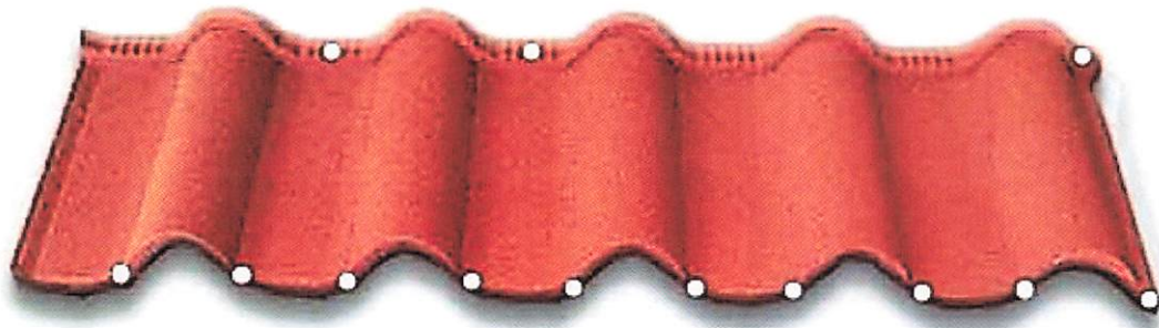
26ga. Steel Mosaic Sicily Tile – 13 fasteners/panel
